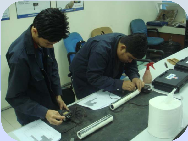
2 UT personnel involved in round robin corrosion measurement project.
