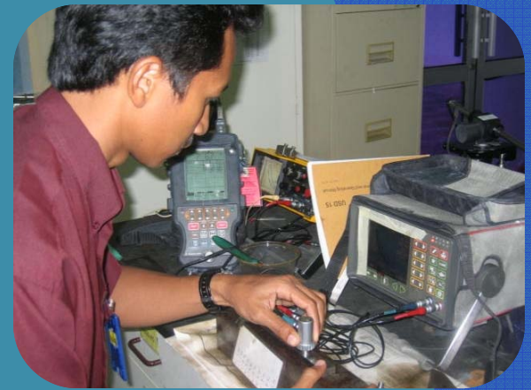
Ultrasonic inspector performing thickness measurement: reliability of data obtained by ultrasonic thickness gauge are questioned by many parties.
